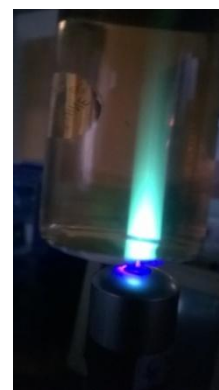
Fig.6 Green emission and blue emission from Si NP solution when excited with a LASER of wavelength 400 nm.
